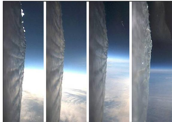
**Figure 4** – BIG BLUE I: Images of deployed wing at 17km, 19.2km, 26.2km, and 27.1km (58k, 63k, 86k, and 89,000ft)
