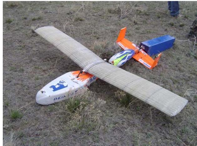
**Figure 5** – BIG BLUE II aircraft and attached inflation system at the recovery site
