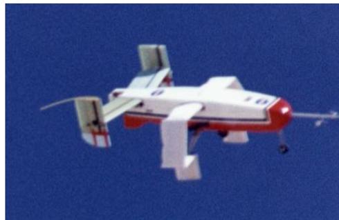
**Figure 2** – NASA Dryden inflatable wing research
