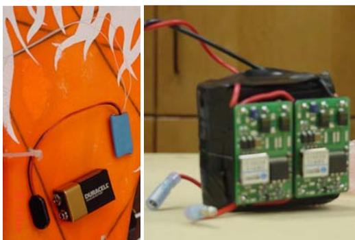
**Figure 7-** BIG BLUE II avionics and control unit (top), beacon (bottom left) and battery pack (bottom right)
