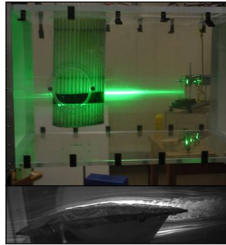
Figure 6 – Wind tunnel testing of the final wing design
